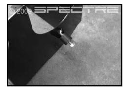
Step 10 Install the rubber mount into the slotted hole in the filter shield. Snug the nut, but do not fully tighten, as you will be adjusting the location in a later step.
