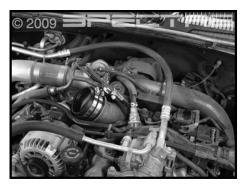
Step 12 Install the coupler on the turbo inlet as shown.
