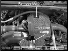
Step 2 Loosen the bolt and remove the stock engine cover or intake resonator (2002 and newer models – must also loosen hose clamp as shown).
