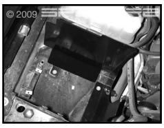
Step 11 Install the filter shield as shown, using 3 of the stock bolts removed in step 8. Fully tighten the bolts.
